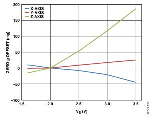
Figure 44. 0 g Offset vs. Supply Voltage
