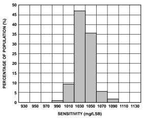
Figure 9. Y-Axis Sensitivity at 25°C,  $V_S = 2 V$ ,  $\pm 2 g$  Range
