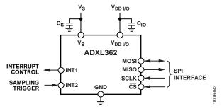
Figure 43. Using the INT2 Pin to Trigger Synchronized Sampling
