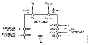
Figure 42. INT1 Pin as the Input for the External Clock
