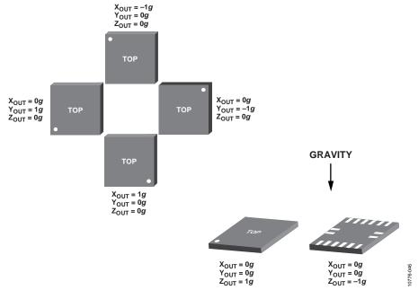
Figure 47. Output Response vs. Orientation to Gravity
