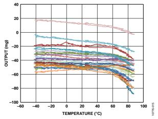
Figure 15. Y-Axis Zero g Offset vs. Temperature— 16 Parts Soldered to PCB, ODR =  $100 \, \text{Hz}$ ,  $V_S = 2 \, \text{V}$
