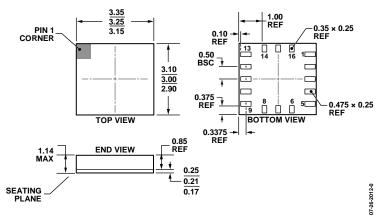
Figure 49. 16-Terminal Land Grid Array [LGA] (CC-16-4) Dimensions shown in millimeters
