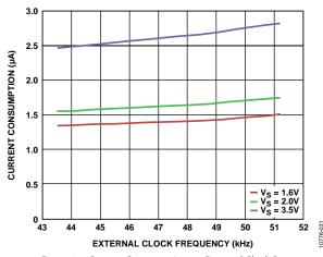
Figure 31. Current Consumption vs. External Clock Rate
