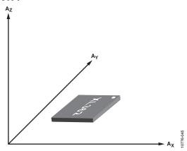
Figure 46. Axes of Acceleration Sensitivity (Corresponding Output Increases When Accelerated Along the Sensitive Axis)
