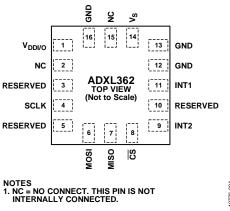
Figure 4. Pin Configuration (Top View)
