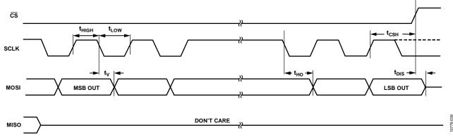
Figure 39. Timing Diagram for SPI Read Instructions
