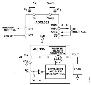
Figure 41. Awake Signal to Control Power to Downstream Circuitry
