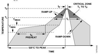
Figure 3. Recommended Soldering Profile
