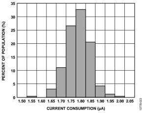
Figure 23. Current Consumption at 25°C, Normal Mode, ODR = 100 Hz,  $V_{\varsigma} = 2$  V
