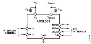
Figure 40. Recommended Bypass Capacitors
