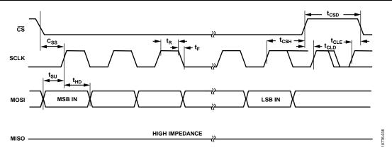
Figure 38. Timing Diagram for SPI Write Instructions
